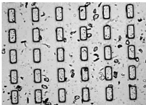
Figure 6a: Stamp that has been soaked in ethanol for cleaning but has not yet been sonicated; note the large amount of material present both on and off the relief surface.
