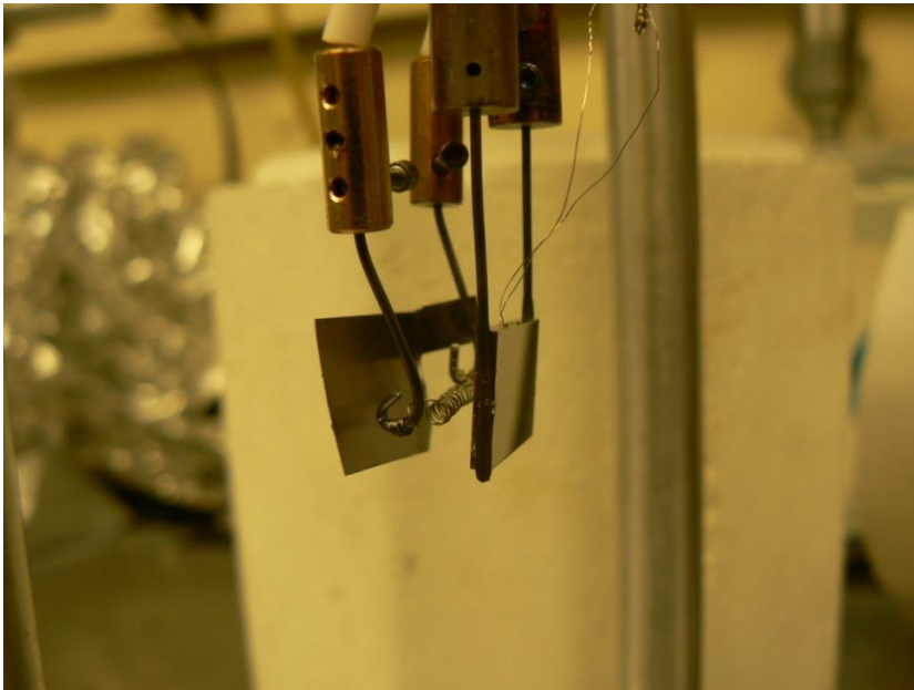
Figure 2. Ruthenium crystal connected to the sample holder by two tantalum wires.
