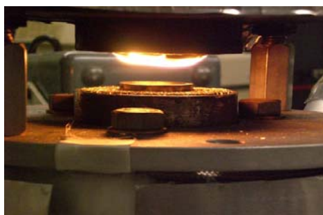
Figure 3: The flame with 50% Oxygen content in oxidizer stream
