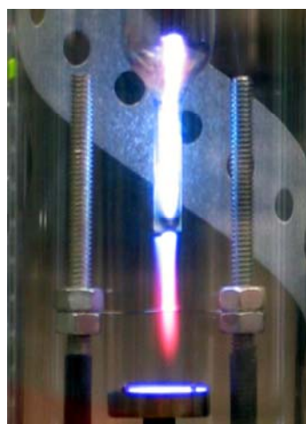
Figure 4: Discharge in ethylene-argon gas mixture
