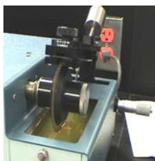
Figure 6. Checking progress on diamond cutting wheel.
