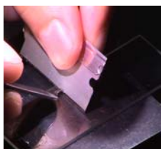
Figure 8. Using razor blade and tweezers to manipulate sample prior to grinding.
