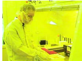
Figure 13. Mike Schaefer soaks a silicone wafer in a developing solution. Yellow lighting is used during the photolithography process.
