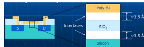
Figure 2. Diagram of cross section of silicon chip and Poly-Silicon transistor. The insulator is SiO 2 , silicon dioxide. (Javier Rosado, 2003)
