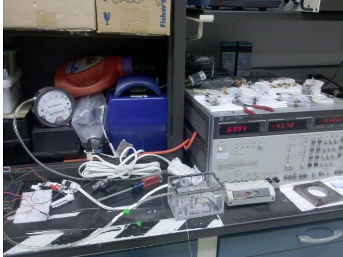
Fig. 6b: Picture of the Experimental Setup Part I for Impedance vs. the Total Pressure
