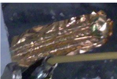
Fig. 1: A pressure sensor. Compliant liquid reservoir is made of Mylar film with a central LDPE tube to place the compliant liquid (saline) into at the middle and LDPE electrodes inserted into the outer edges of the film.
