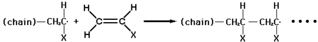
Figure 2 – Formation of polymers: the propagation reaction
