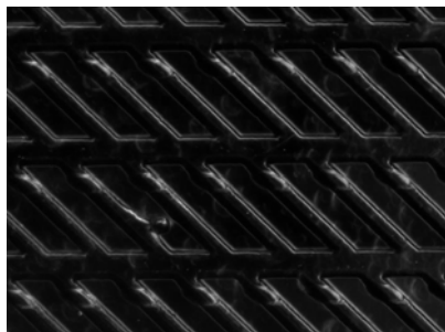
Fig.5-a – ‘Control’ image of device used to cancel out interference caused by PDMS mixer pattern.
