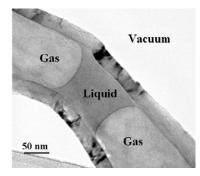
The adjacent figure shows a transmission electron photomicrograph of an elbow portion of a capped carbon nanotube made hydrothermally [15]. The tube contains a liquid inclusion constrained between two menisci separating the aqueous liquid from the adjoining gas. The nanotube rests on a holey carbon grid, a segment of which is visible in the lower left corner of the micrograph. The volume of the liquid inclusion is of the order of  $10^{-18}$  (*atto*) liters.
